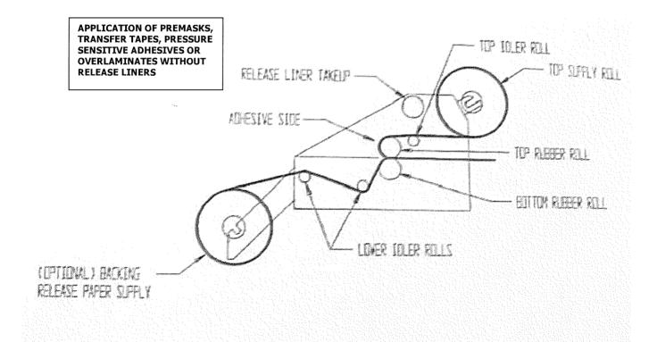
NOTE: The operator rust use a backing paper either from a supply roll or in sheets to prevent achesive from adhering to the machine
