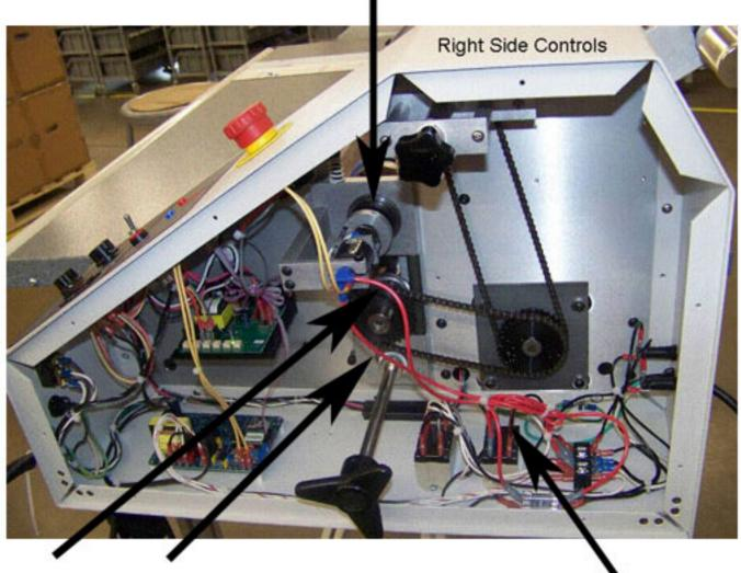
If the heat relay clicks there should be 110 volts to these two red wires. If there is, either the rotary connector is bad or the heater is bad. Check the inner 2 heater wires for continuity. If OK, then replace the slip ring. If no continuity, the heater cartridge is bad.
