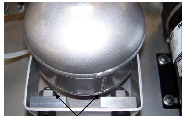
AIR TANK MOUNTING BRACKETS/ EXCESS INWARD
