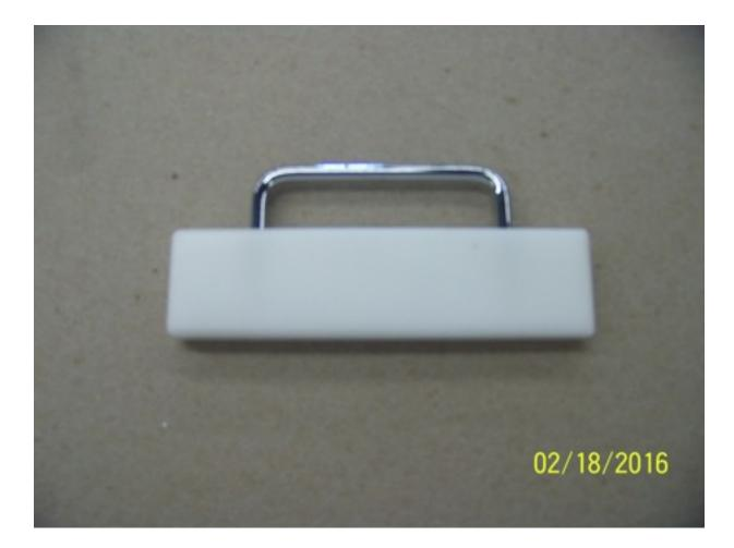
**Gap Gauge Block**-Used on old style EP series machines to set the roller gap for 1" thick materials. It is a 5/8" thick piece of Delrin plastic and handle. There were 2 sent with each machine
