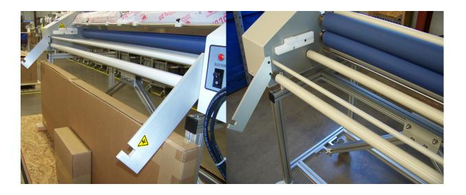
SUPPLY ROLL KIT: 2<sup>ND</sup> COMPLETE SUPPLY ROLL WITH STOP COLLAR, REPLACE LOWER STABILIZER WITH IDLER TUBE COMPLETE, & (2) FRONT SUPPLY ROLL BRACKETS. SECURE BOTH WITH 1⁄4 -20 X 3⁄4 BHSH.
