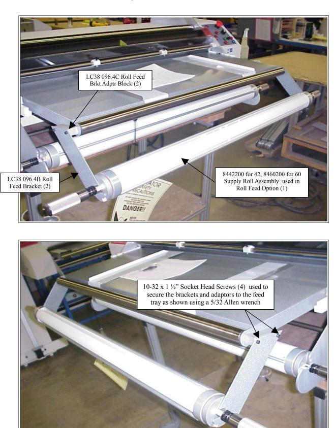
Assembly part #'s for the Roll Feed Option are 8342500 for D42 and 8360500 for D60
