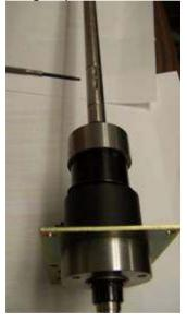
When installing a clutch on a new shaft you simply align the clutch and the woodruff key grooves and then drill and pin it.
