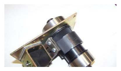
Before you put the snap ring back in its groove, cycle the clutch several times to make sure it stops at the proper position
