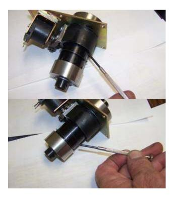
Slide the concentric ring towards the chrome hub of the clutch until it is totally off of the splined part
