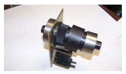
You can now rotate the clutch until the keyways are in the straight up position.
