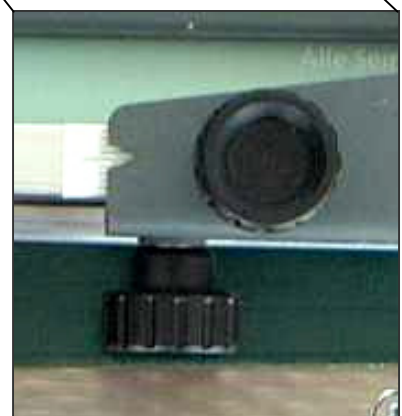
detail 2 Micro adjustment for the infeed angle
