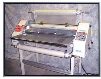
2. Slide a roll of film onto the top supply roll mandrel. Center the roll on the mandrel and place the mandrel in the top bracket. This is a job best done with two people, even if the roll of film is not very heavy. With a person holding each end of the mandrel, it is easy to put both hexagonal fittings into their respective brackets. Make sure they are both fully seated. Attempting to load the film on the laminator by yourself may result in a back strain or other injury.
