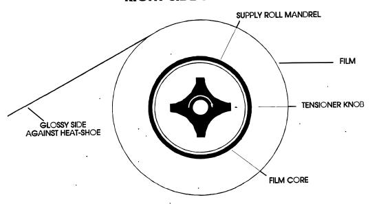
2. Slide a roll of film onto the top supply roll mandrel. Center the roll on the mandrel and place the mandrel in the top bracket. Make sure the dull side of the film is facing up and the shiny side is facing the heat shoes during the threading.
