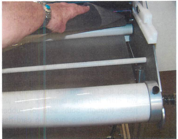
Bottom film under support shaft & idler
