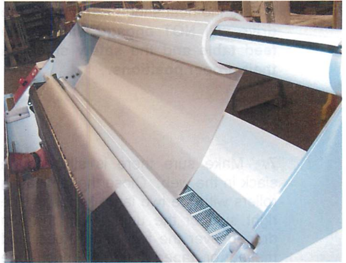
Top film under idler, over S-wrap, onto shoe
