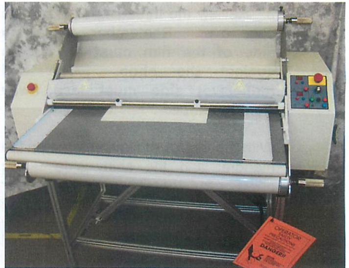
With rubber rolls locked down, thread film
