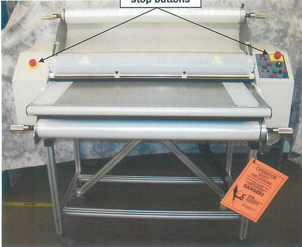
Emergency stop buttons
