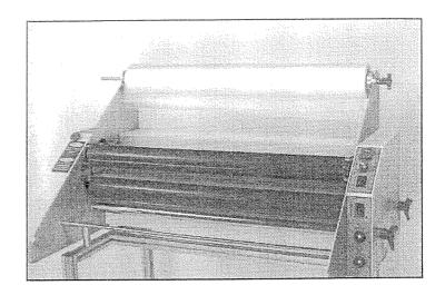
5. Review the threading diagram one page over. Run the film from the top mandrel and drape it across the top heat shoe. Remember, the shiny side of the film must always go against the shoe. The dull (adhesive) side must face away from the shoe. With the top roll of film centered on the mandrel and the shiny side facing down and draped over the top heat shoe, you are now ready to load the bottom supply roll mandrel.
