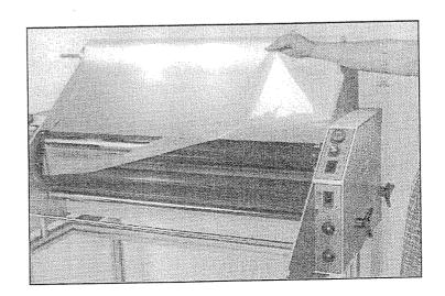
4. Center the roll on the mandrel and place the mandrel in the top brackets. This is a job best done with two people, even if the roll of film is not very heavy. With a person holding each end of the mandrel, it is easy to put both hexagonal fittings into their respective brackets. Make sure they are both fully seated. Attempting to load the film on the laminator by yourself may result in a back strain or other injury.
