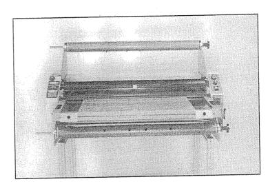
3. Slide a roll of film onto the top supply roll mandrel, turning the roll slightly to slide the gripper inside the core. Center the roll. Make sure the dull side of the film is facing up and the shiny side is facing the heat shoes during the threading.
