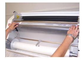
5. Rotate the film supply sensor until it touches the film roll. Pull about 18 inches of film from the bottom roll, and drape over the rollers.
