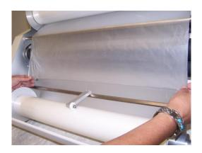
6. Pull a length of film from the top roll. Drape it over the top idler bar and across the rollers.
