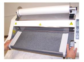
8. Depress the feed table latches and reinstall the tray. Push it in firmly until the front edge is flush with the front of the machine. NOTE: If the tray is not fully engaged, you will see a small wrench on the display screen.
