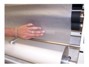
7. Tape the two pieces of film together with cellophane or masking tape. This is just to hold the rolls of film together during the threading process.
