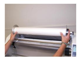
4. Place the film rolls in the slots in the side panels of the machine
