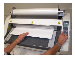
9. Set the desired laminating temperature and allow the machine to heat up. When the hourglass symbol goes out, the machine is ready to laminate. Place the feed card on the feed table and push in firmly while pressing the forward motor control button. Feed the card all the way through the machine. NOTE: After initial threading, it will be necessary to run 2-3 feet of film through the machine before the laminate smoothes out.
