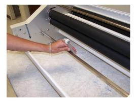
2. Lift film supply sensor to a straight up position.
