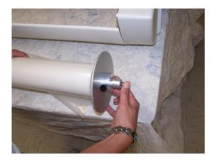
3. Load film onto supply rolls. Center the film, and lock it into place using the supply roll retainers.
